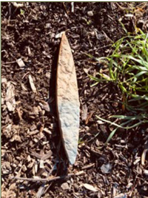
This curved sharpening stone is made for a scythe, but can be used with any medium to large, curved blade
